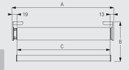
A: system width (inside recess includes bracket covers) B: system drop C: fabric width
