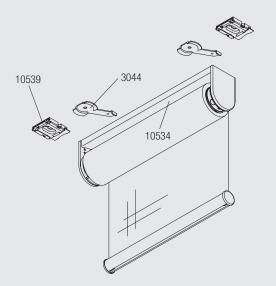
System is pre-mounted on continuous installation profile 10534 for fast fitting on site. Just mount the system with pre-fixed clamps 3044 or click brackets 10539.
