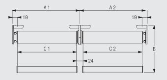
A: system width (inside recess includes bracket covers) B: system drop C: fabric width
