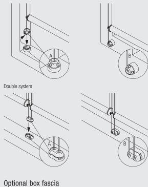
A: Fitting of side guides inside window frame B: Fitting of side guides to front of window frame
