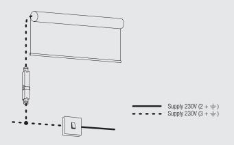
Operation with Radio Remote Control System 9940 or 0450
