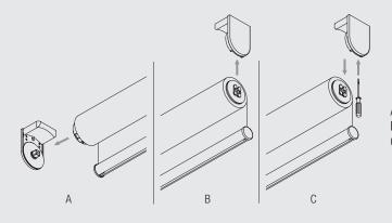
A: Insert roller blind into support bracket (drive side) B: Click roller blind into support bracket (click side) C: Use small screwdriver to remove roller blind
