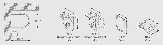
All measurements are based on the maximum system dimensions.
