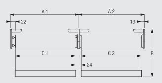
A: system width (inside recess includes bracket covers) B: system drop C: fabric width
