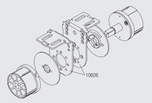
The optional centre support bracket allows two connected systems to be powered by one motor. It can also be combined with continuous installation profile for easy on-site fixing.
